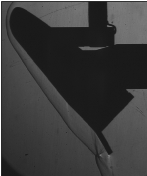
Fig. 19 CFD visualization (left) and schlieren picture (right). M = 14 , \alpha = 45 deg, \delta_e = 15 deg conditions.
